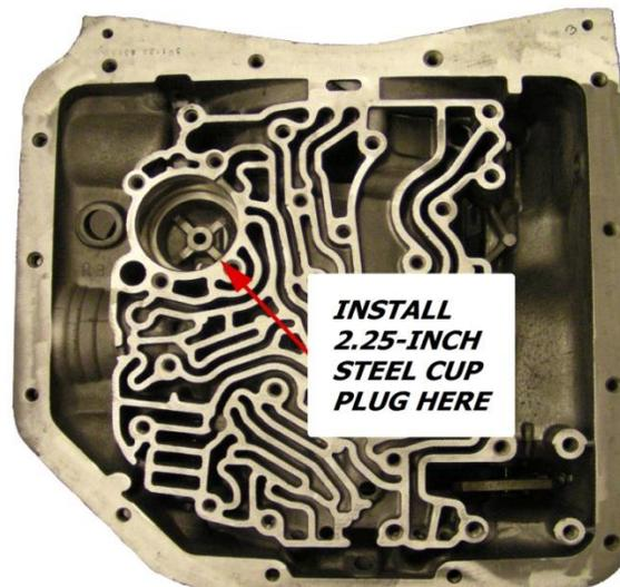
15. Install new upper valve body gasket, new separator plate, and new lower valve body gasket onto transmission case. Install support plate to hold gaskets and separator plate in place. Only hand-tighten the support plate bolts. DO NOT tighten support plate bolts completely until valve body has been installed onto transmission.
